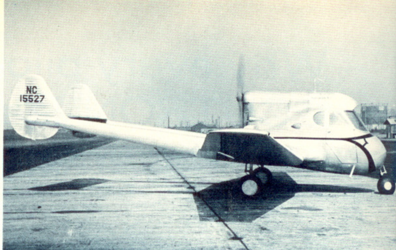
Stearman-Hammond Y-1S, with air scoop for inverted Menasco engine above windshield. Its advanced structural features included crimp-corrugated control surface skins which are the standard today
